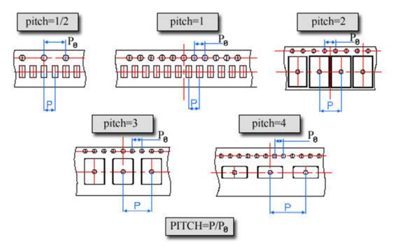
It can be seen that pitch equals the number of puncture holes between two parts (gaps between two holes are 4mm on all tapes). **PRESET** key: Press this key and enter the desired number. The machine counts to this preset number and stops. Pressing the key again will return to normal mode.
